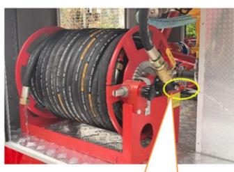
Pump Drain Ball Valve: To discharge all water inside the fire pump
